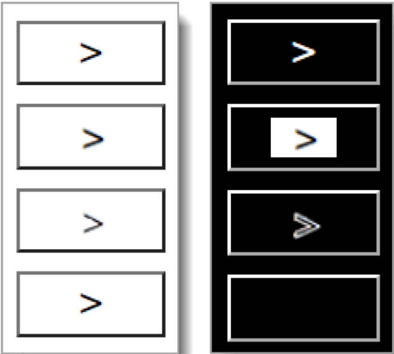
Figure 8: Four icon buttons in the default presentation (left) and with the use of Windows Contrast Adjustment (right).
